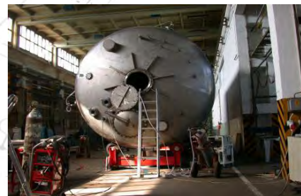
On-site special leak testing
